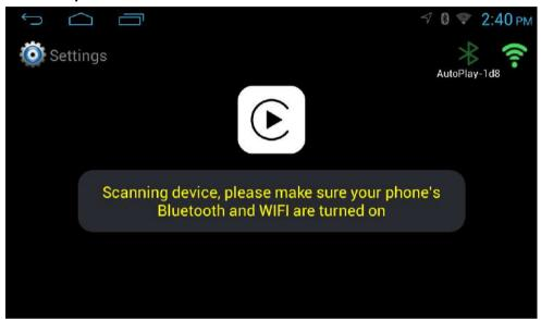
6. Open IPhone Bluetooth and WIFI function, looking for the Bluetooth AutoPlay-XXXX device number, pairing code: 0000 (The first connection to the Bluetooth needs to be manually paired, and it can be automatically paired afterwards) (Wireless CarPlay connection mode: Bluetooth is a pairing function, Bluetooth is automatically disconnected after successful pairing. WIFI is used to transmit data, so you need to open IPhone Bluetooth and WIFI function.)
