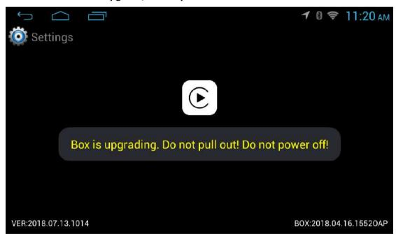
9. After the upgrade of the box is completed , the phone can be inserted again to use the function .
