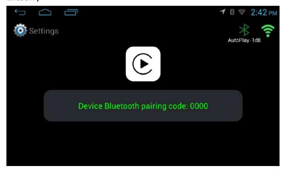
5. Open IPhone Bluetooth and WIFI function, looking for the Bluetooth AutoPlay-XXXX device number, pairing code: 0000 (The first connection to the Bluetooth needs to be manually paired, and it can be automatically paired afterwards) (Wireless CarPlay connection mode: Bluetooth is a pairing function, Bluetooth is automatically disconnected after successful pairing. WIFI is used to transmit data, so you need to open IPhone Bluetooth and WIFI function.)
